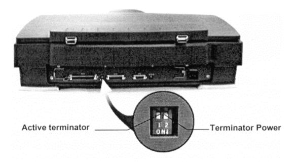
In this situation, the card will have a built-in terminator. The card forms one end of the SCSI chain; the scanner forms the other end. Turn on the "active terminator" and "terminator power" switch by pressing them down to enable the built-in "active terminator" function. These will ensure that there are two terminators and that they are placed at the ends of the SCSI chain.
